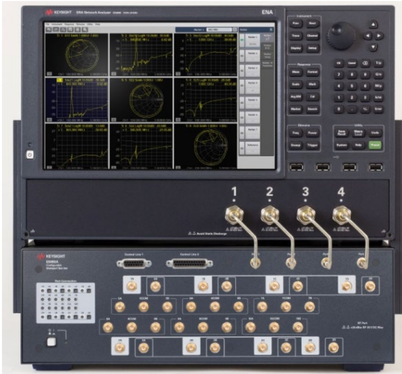
Figure 1. Multiport setup using the E5092A
